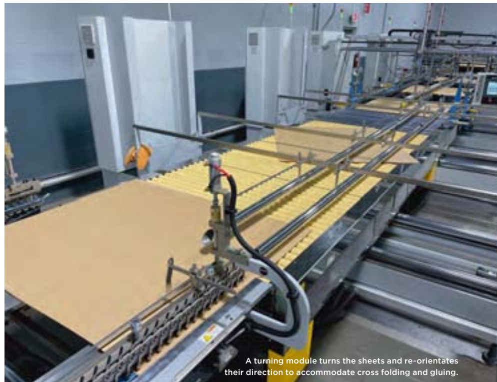
The specialty gluer is 10 ft wide and can easily handle sheets as large as 118 inches.
