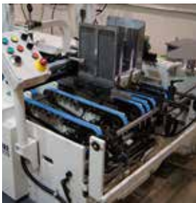
High Performance Feeder Section for accurate carton spacing. Servo motor drive allows for precise spacing out of the feeder. Vacuum and vibrator belts come standard.
