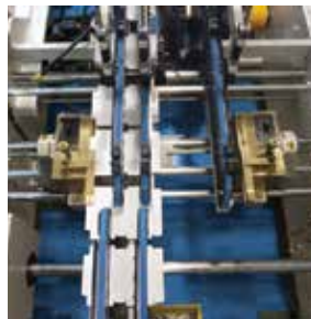
Left and Right Glue Pots are standard for gluing A&B style cartons and adding more versatility. Various width glue wheels available, knurled or smooth.
