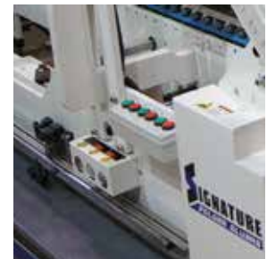
Motorized Carriers with digital indicators for precise and easy make-ready on repeat jobs.
