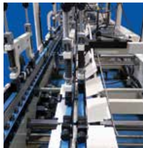
Versatile Pre-Break Section for 180-degree first-and third-score prebreak and compound folding options. Includes an extended-height third score pre-break area for large cartons.
