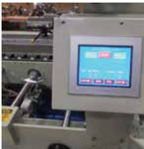
4&6 Corner Servo Backfold System for reliable 4&6 corner productivity. Touch screen control adjustments can be made on the fly without the need for shaft reconfiguration.
