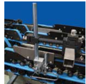
Crash-Lock Bottom Attachments designed as a single-clamping system that can be preassembled and quickly positioned to reduce set-up time.
