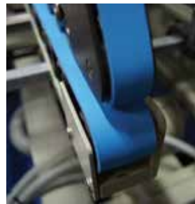
Offset Carrier Belts for strong blank support along a score line, accomplished with lower carrier belts that are wider than the top.
