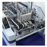
High Performance Feeder Section for accurate carton spacing. Servo motor drive allows for precise spacing out of the feeder. Vacuum and vibrator belts come standard.
