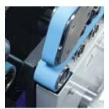
Offset Carrier Belts for strong blank support along a score line, accomplished with lower carrier belts that are wider than the top.
