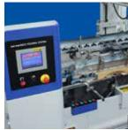
4&6 Corner Servo Backfold System for reliable 4&6 corner productivity. Touch screen control adjustments can be made on the fly without the need for shaft reconfiguration.
