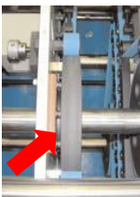
Grease pulley guides every 3 months. Machine must be turned off and disconnected from power. Take safety guard off to lube. Make sure to replace safety guard when finished.
